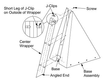
Figure 3 - Attaching Center Wrapper to Base Assembly
